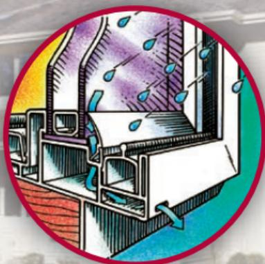
*Windows and doors often have a simple drainage system or “weep” system designed right into the product. These water drainage pathways must be kept clear and clean for the window or door to operate correctly.*
